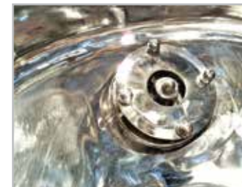
Bottom Mounted Homogeniser provided with Rotar & Stator
