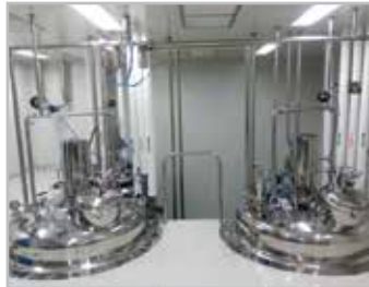
All wetted Parts of SS 316(cGMP Model) & pipelines are electro-polish from inside
