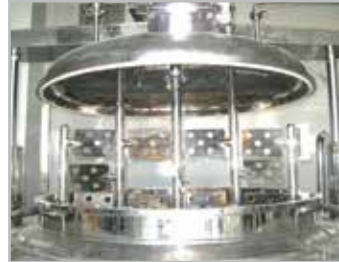
Complete hydraulic lid lifting arrangement with safety interlock.
