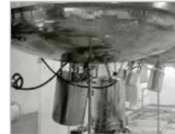
Bottom entry Angular CROWEL TYPR IMPELLER for Uniform mixing.
