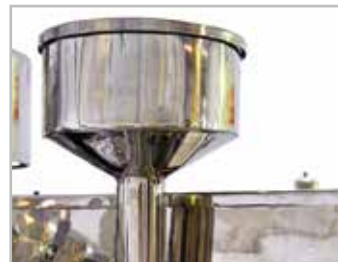
Provided with Addictive Hopper for adding Active Ingredients
