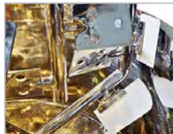
Provided with Teflon Scrappers, floating type, self adjustable for Complete scrapping of vessel
